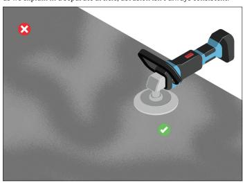
There are several other methods of surface preparation you can use to remove contamination. Abrasion is usually the 'go-to' method. Even if it isn't always the best. Regardless of contamination and abrasion, there's one thing that ultimately determines a material's ability to form a strong bond – surface energy.
