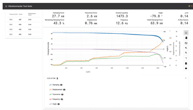
Figure 1: Junker test loosening curves demonstrate self-loosening behaviour, providing valuable data for fastener performance comparison but not bolted joint performance
