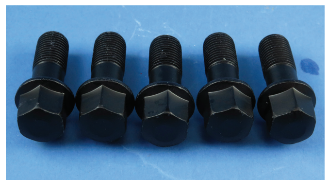
Picture 5b: ZnNi + passivate + sealer + Techseal® Black SL
