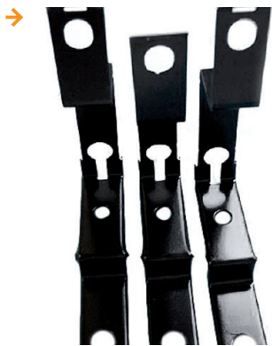
Picture 6: Zinni® AL 450 S + EcoTri® NC + Zintek® Top Black S after >1,000h in NSS/ISO 9227
