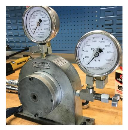
By applying the specified torque to the bolt in the load cell, you can mimic the bolted joint as closely as possible and see how much tension is developed
