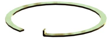
The bent end offers a 'nose' which hinders the rotation. No additional keystone needs to be handled in the assembly process. Time and costs for machining the additional groove is comparatively less.
