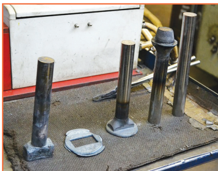
Figure 1 – bolt head hot forging sequence from right to left (courtesy of Smith Bullough Ltd)
