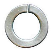
Split lock washers, as we know it, are strength wise only capable to withstand clamp forces introduced by fasteners up to property Class 5.8 (when using the fasteners full potential). When used with these fasteners split lock washers will reduce the loss of clamp load thereby reducing the risk of loosening due to dynamic forces. Also most split lock washer's edges will create a mechanical locking onto soft surfaces that will improve the locking effect.
