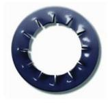
**Ribbed lock washers:** Ribbed lock washers are ridged at least on one side. Together with the friction in the thread, the friction in the bearing area prevents spontaneous rotational loosening of screws and/or nuts by considerably increasing friction between the bearing areas.
