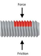
If the screw revolves when applying the coating, a 360° polyamide coating is formed. This does not only jam, but it simultaneously seals the thread – which is important in screws that are designed to seal containers. The polyamide coating can be directly applied to the area where it has to be effective, i.e. where the external/internal threads are engaged. The thickness of the
