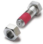
Friction is maintained and the screws/nuts are vibration resistant. Full hardening can take up to 72 hours, but in most cases the part is already locked after a short period of time. Therefore adjusting the fasteners after assembly should be avoided as that can damage the locking effect.
