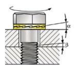
Nord-Lock®: A special serrated locking washer is the Nord-Lock® washer. These always come as two washers paired together to provide the locking effect. The outer surfaces are ribbed and will bite into even the hardest materials, while the inner surfaces have precision ground ramps.
