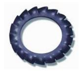
Serrated lock washers: The name serrated lock washers is misleading. These washers only function is to promote electrical conductivity. These are often used on grounding applications such as for car batteries. The twisted teeth of the washer may appear to be a locking feature, but the reality
